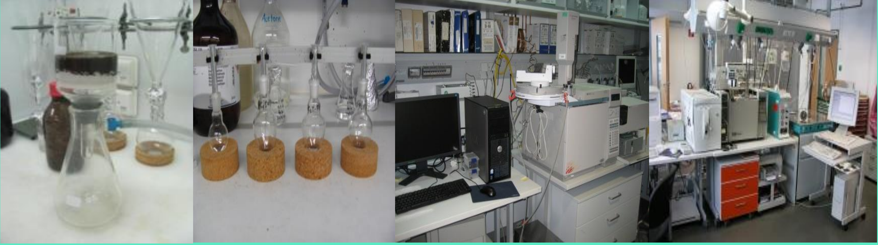
Fig. 6 PLFA and NLFA extraction and measurement in GC-FID and GC-IRMS systems
